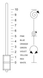
In the 0% to 50% range of adjustment the colour change in response to movement of the potentiometer is linear and continuous so that the slider can be stopped in intermediate positions to obtain a two-colour beam.
