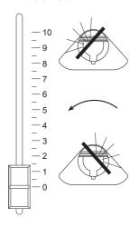
Horizontal movement (Pan) of the mirror occurs gradually as the slider is advanced. From the zero position mirror movement is linear and continuous up to the opposite end of travel. The mirror can be stopped at any intermediate angle.
