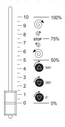
From 0% to 49.7% the gobo rotates through 540° (1  $^{1/2}$  turns).
