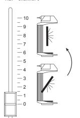
Vertical movement (Tilt) of the mirror occurs gradually as the slider is advanced. From the zero position mirror movement is linear and continuous up to the opposite end of travel. The mirror can be stopped at any intermediate angle.
