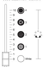
The change occurs instantaneously as the slider reaches different preset levels on the graduated scale.
